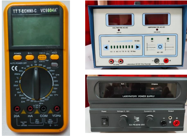
Figure 1.2 Digital measuring instruments used in the laboratory; digital multimeter and power supplies.
