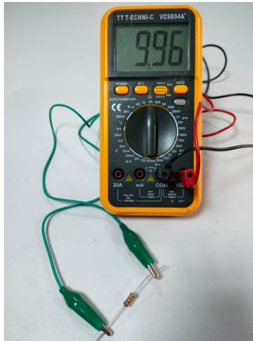
Figure 1.4 Measuring resistance value with a digital multimeter
