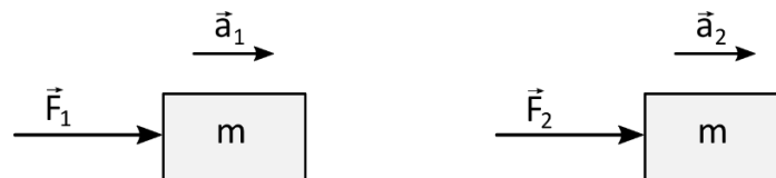
Figure 7.2 The effect of different forces \vec{F} applied to two objects of the same mass on the acceleration.
