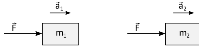
Figure 7.1 The effect of a constant force \vec{F} on the acceleration of two objects with different mass.
