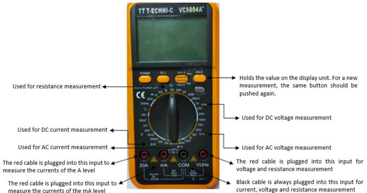
Figure 1.3 Usage of the digital multimeter
