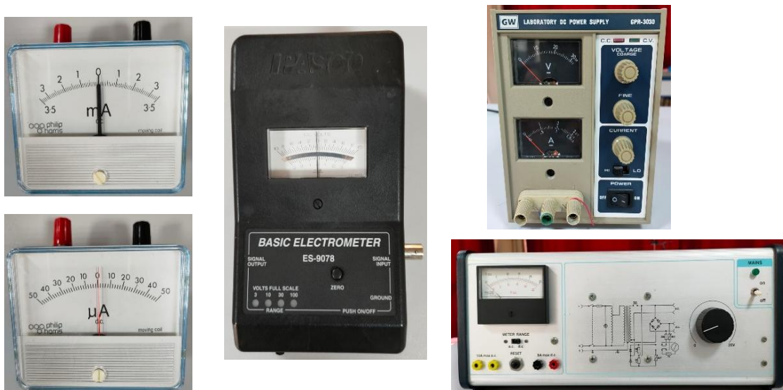
Figure 1.1 Analog measuring instruments used in the laboratory; milliammeter, microammeter, electrometer and power supplies.
